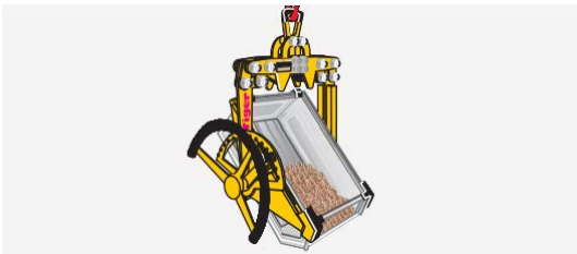
Fig. 9-2 Box gripper for emptying
