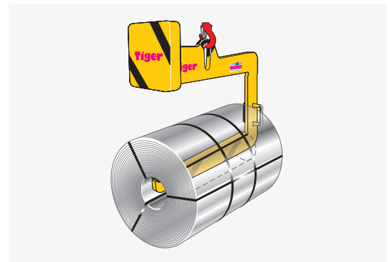
Fig. 26-3 C-hook with counterweight
