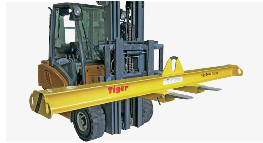
Fig. 25-1 Stacker with girder-type beam
