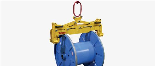
Fig. 9-5 Coil gripper
