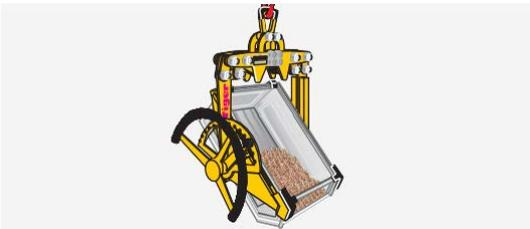
Fig. 9-2 Box gripper for emptying
